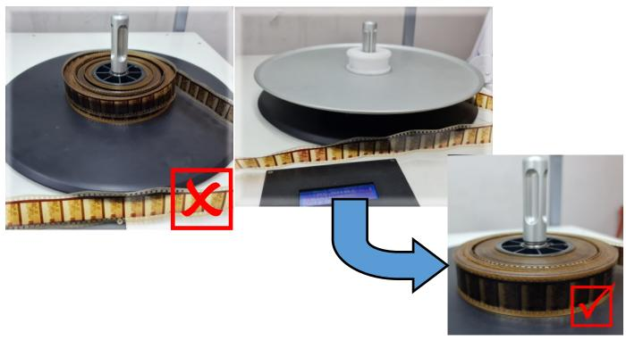
Pressure plate can be also, as secondary use, an aid in simplifying the handling of soft and loose film reels.
