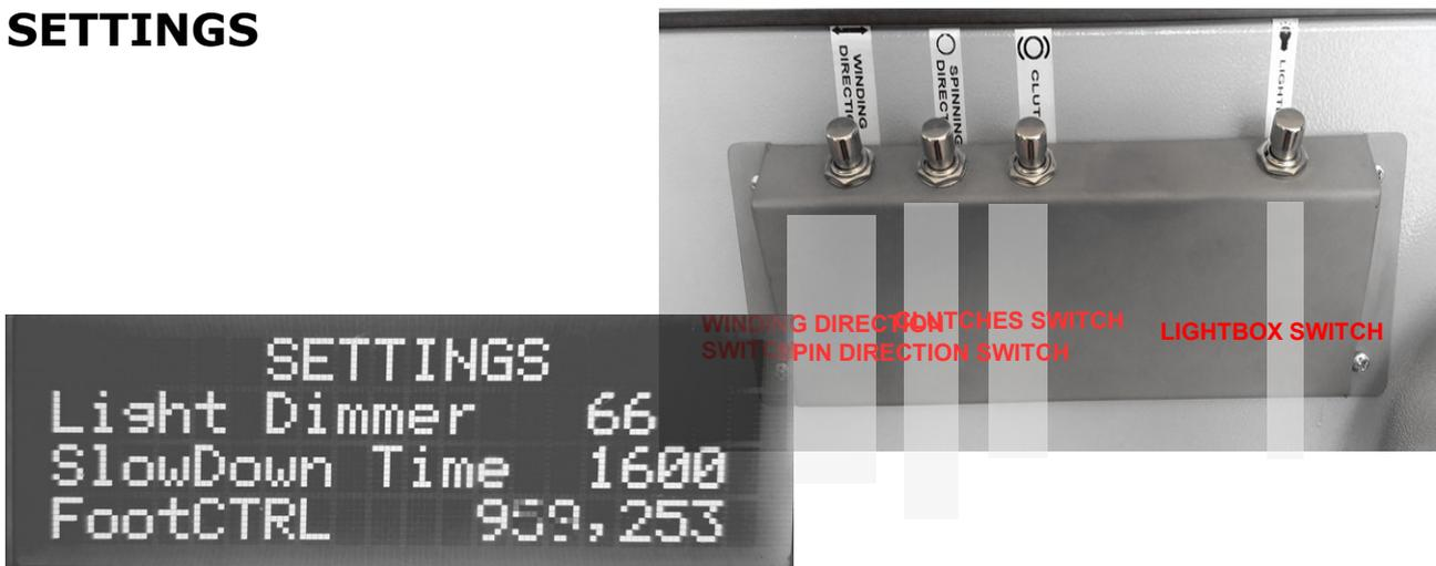
To get **access** to the setting menu, keep the *lightbox switch button* pressed when switching on the equipment.
